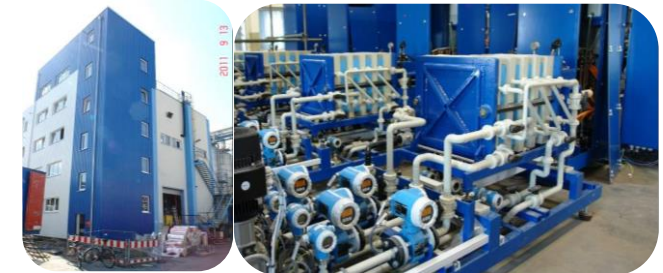
Pilot plant for conversion of Li-salts to LiOH Bg
